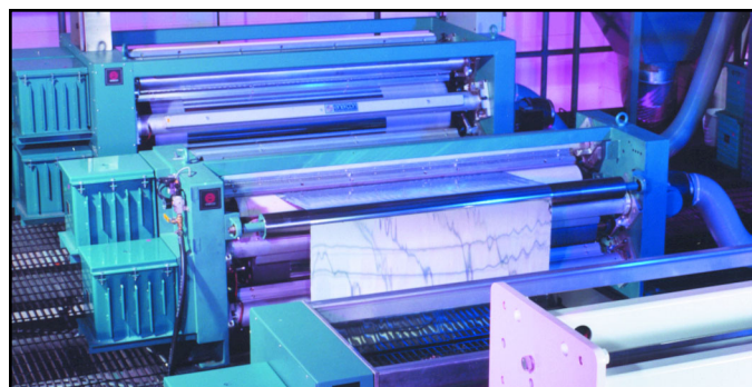
Enercon's lab features corona, plasma and flame treating up to 60" wide and 1,000 fpm .
